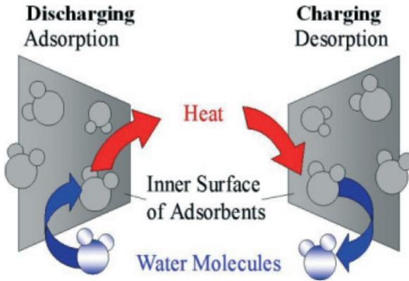
*Figure 5 – TES De/Adsorption Process*
