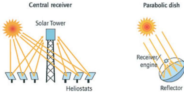
**Figure 3 – Solar Tower and Solar Dish Concepts**
