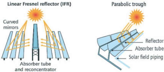
**Figure 2 – Parabolic Trough and Fresnel Reflector**
